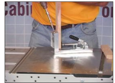
STEP 4: Use Sommerfeld's 3-in-1 Pocket Cutter or pin the frame together
